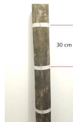
Figure 03: Log piece with rubber band every 30 cm, ready for scanning.
